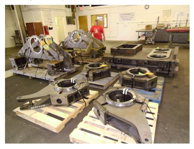
Fabricated & Machined Components for Construction Machinery
